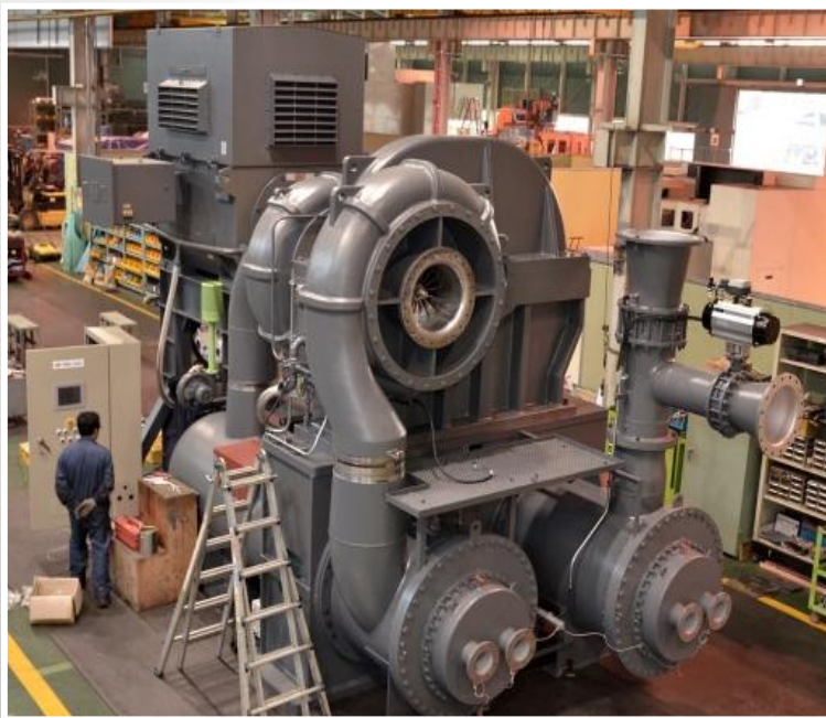
5000HP Air Compressor
